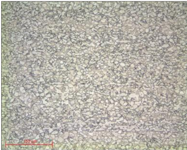
Micrograph 12: TA6V untreated Kroll lens x20 TA6V reagent etched
