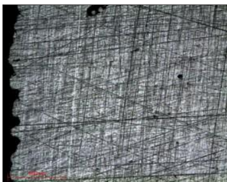
Micrograph 1: Surface condition P320 lens x5
