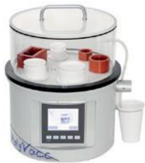
Fig 6: Vacuum mounting device: POLYVAC
