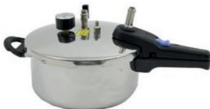
Fig 5: Pressurized mounting device
