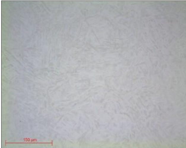
Micrograph 10: TA6V polished up to SPM lens x20
