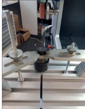
Figures 15 & 16: Examples of clamping and electronic connector 4000 series wire saw
