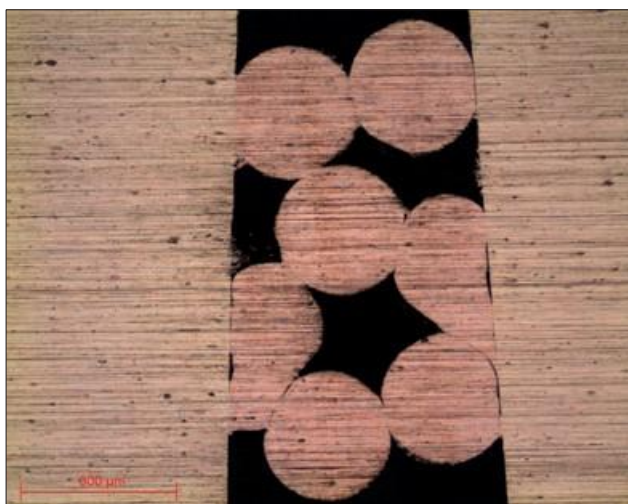
Micrograph 1: Polished crimp up to 3µm lens x10
