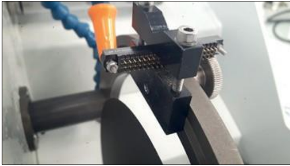
Figure 14: Example of clamping a connector MECATOME T202
