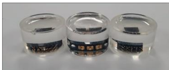
Figure 19: Coating with the use of "pressure coating equipment"
