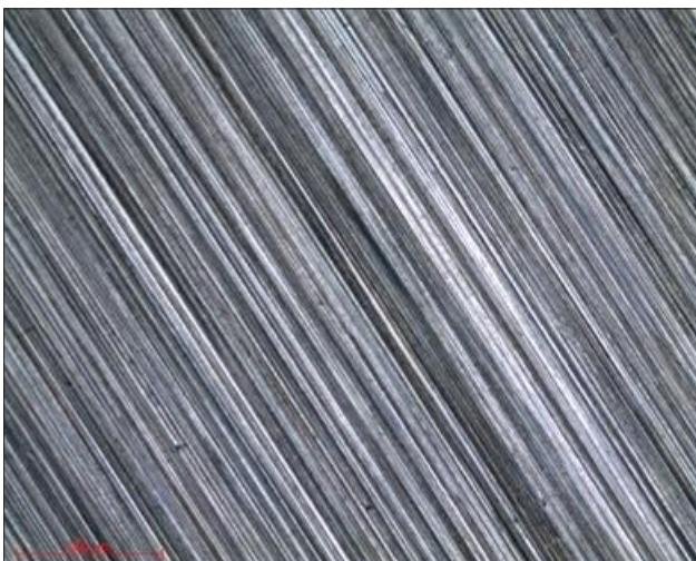
Micrograph 1: Surface condition P320 lens x5
