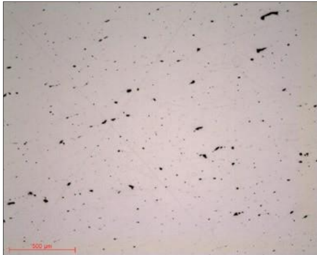
Micrograph 3: Surface condition RAM 3µm lens x5
