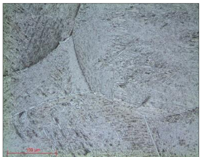
Micrograph 18: Titanium etched with KROLL reagent lens x20
