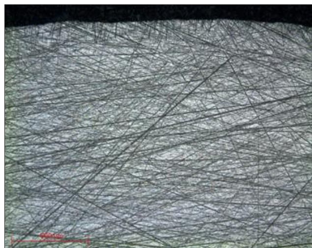
Micrograph 9: Surface condition TISSEDIAM 20μm lens x5
