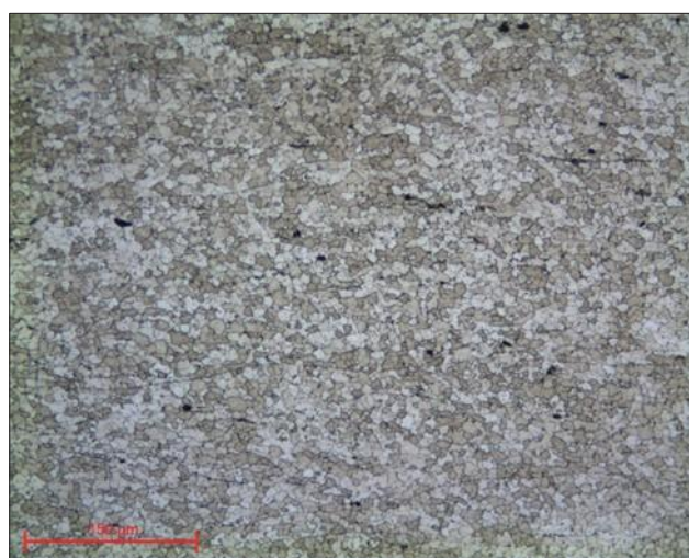
Fig. 29: Structure Aluminum lensx20
