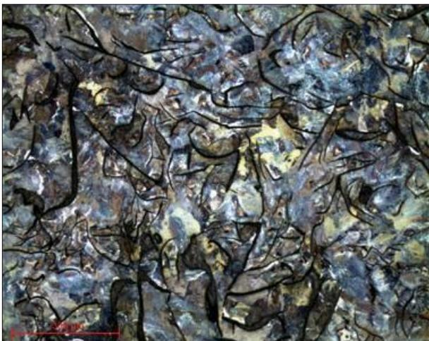
Fig. 19: Cast iron GL core lens x10
