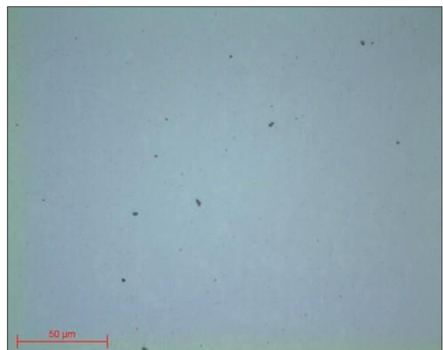
Micrographs 15 and 16: Stainless steel polished up to Al 2 O 3 N°3 lens x10 and x50
