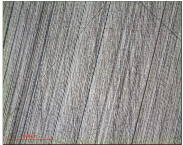
Micrograph 7: Surface condition I-Max R 18µm lens x5
