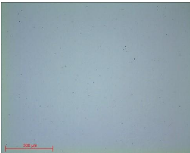
Micrographs 15 and 16: Stainless steel polished up to Al 2 O 3 N°3 lens x10 and x50
