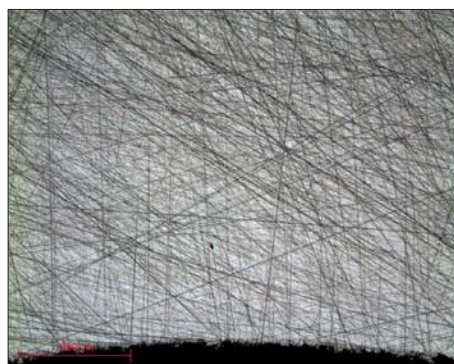
Micrograph 11: Surface condition MED R 9µm lens x5
