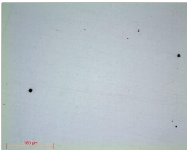
Micrographs 17 and 18: Stainless steels polished up to Al 2 O 3 N°3 lens x20
