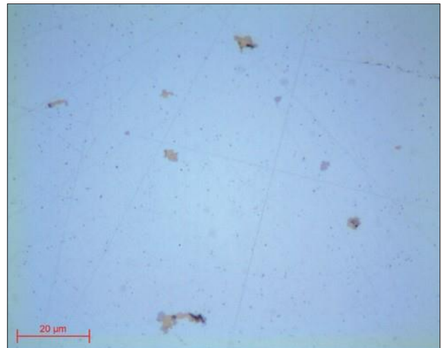
Micrographs 13 and 14: Stainless steel polished up to 1μm lens x20 and x100
