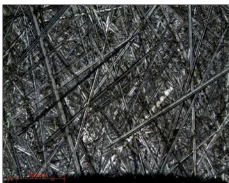
Micrograph 10: Surface condition P80 lens x5
